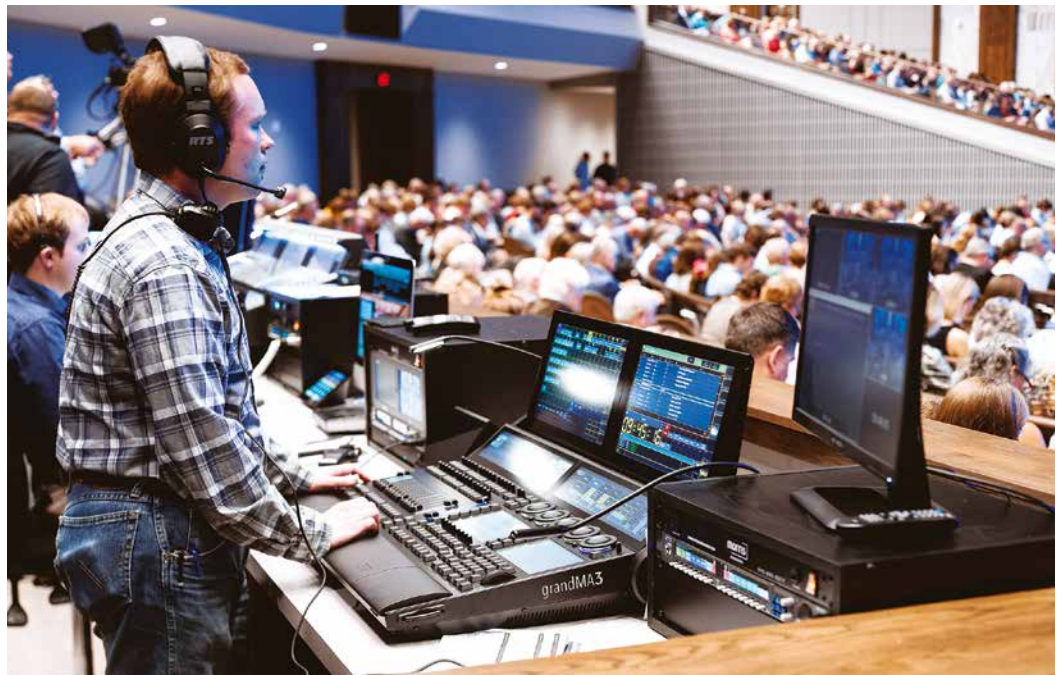
A grandMA3 light console provides 60 physical playbacks
